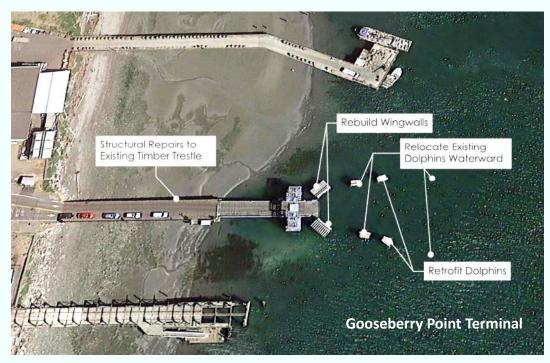
The new ferry is wider and longer than the Chief so the ferry slips on both sides will have to be widened and extended.
